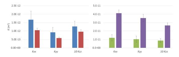
**Figure 3:** Permeability measurements for carbon (left) and glass (right): bag tool = left column of each pair, rigid tool = right.
