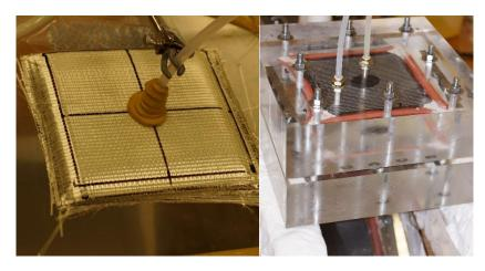
Figure 1: Permeability measurement tools: vacuum bag (left) and rigid (right).
