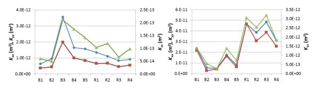
**Figure 2:** Permeability measurements for carbon (left) and glass (right):  $\blacklozenge = K_{xx}$ ,  $\blacksquare = K_{yy}$ ,  $\blacktriangle = K_{zz}$ .
